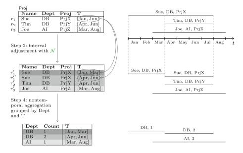
Fig. 13. Illustration of temporal normalizer for a temporal aggregation query.
